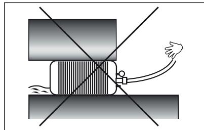
**Pipe stoppers** are made of quality rubber reinforced with nylon or kevlar fabric. The metal parts are made of stainless materials. Each pipe stopper is provided with quick coupling for inflation and eyebolt for removing and blocking. They withstand weather, temperature from -30 °C to 80 °C, use and waste water and they are middle resistant of chemicals. They are mainly used during repair and maintenance works, accidents and for the leak tests with water or air.
